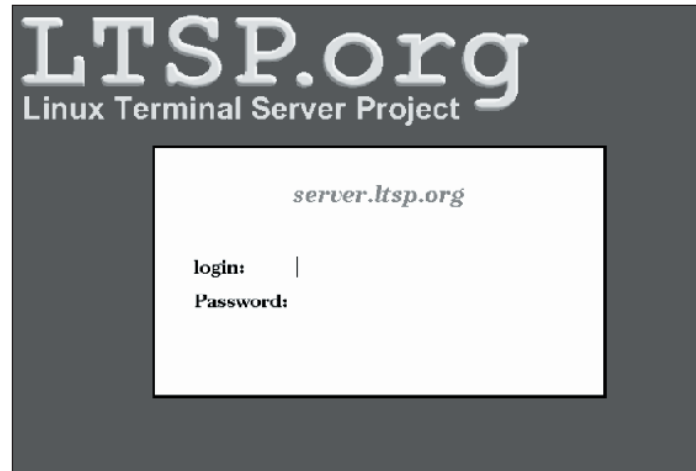
LTSP uses XDMCP to give remote login capabilities to the machines connected to the server via the LAN.
