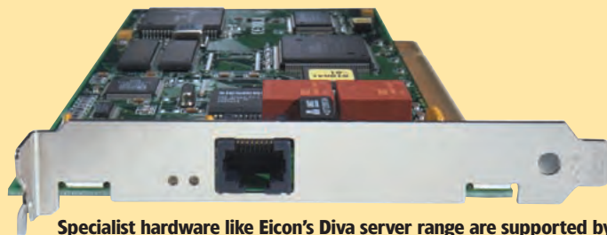
Specialist hardware like Eicon's Diva server range are supported by the kernel and provide interconnectivity with a variety of comms systems such as ISDN, SDL, GSM and analogue voice calls.
