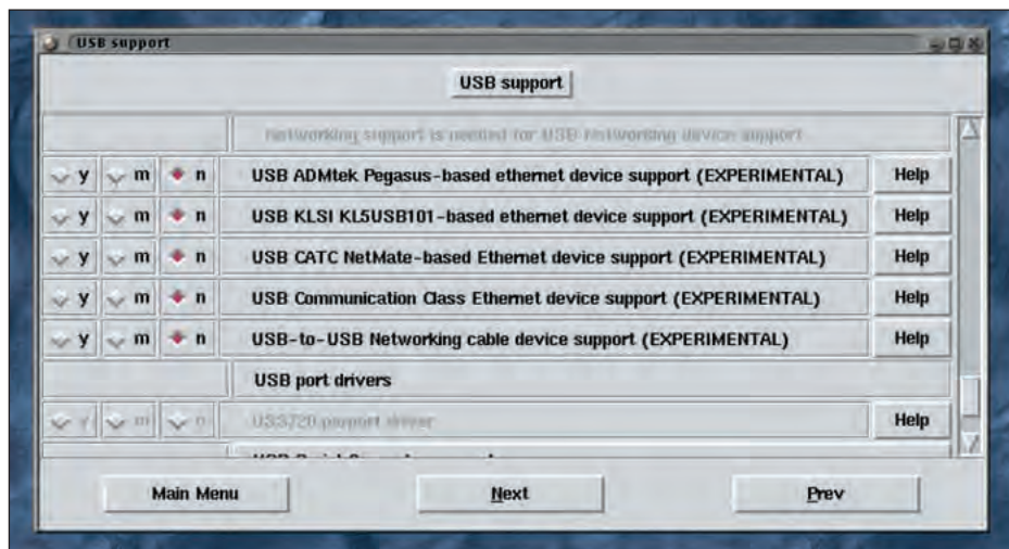
Linux's USB sub-system can support a number of different Ethernet chipsets, but you need to know which one to use, find a list of drivers at http://www.linux-usb.org/
