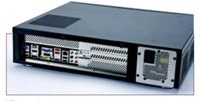
The case we've chosen will only fit a micro-ATX board. This is a form factor several revisions smaller than standard ATX.
