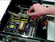
2 Fit the motherboard Orientate the motherboard so the holes in the board line up with the spacers on the case. Don't forget to fit the backing plate provided with the motherboard (as we did, only to realise the mistake much later), and screw a flat screw into each motherboard hole.
