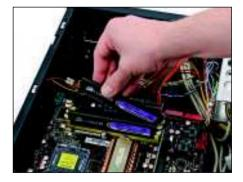
3 Memory and connectors Use the header description in the motherboard manual and the labels on each wire to connect each one correctly to the motherboard. Snap together the wide and square power connectors, attach this, and then slot in your memory modules.
