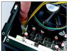
Connect fan and power > Rotate the fan so that the power connector can attach to the motherboard, and place it
