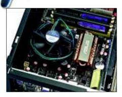
Attach the CPU Unlatch the CPU socket on the motherboard
