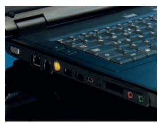
The Znote's has connector for FireWire, modem, Ethernet and VGA, as well as a multimedia card slot and four USB ports.
