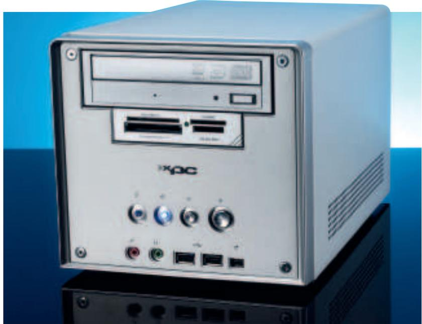
» The Shuttle LinuXPC is small and quiet, but this means that it has limited upgrade potential – you're never going to fit a powerful graphics card into that small box.
