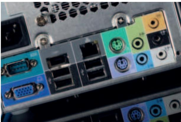
» A card reader, two USB ports and a mini-Firewire port on the front complement the Ethernet, four USB ports, standard Firewire, PS2 and audio ports on the back of the LinuXPC.
